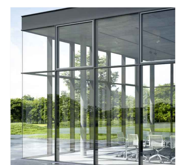
03 - Schuco FWS50 Aluminium glazing facade system or equiv. in dark grey with solar control double or triple glazing. Frame system target u-value of 0.9W/m 2 K or better
